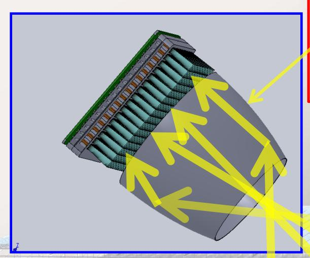
A secondary concentrator properly designed can redirect rays from the collector perifery and spread them more evenly into the TIR prisms.
