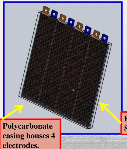
Electrolyzer Single Panel 9 total Electrolyzer Panels bundled to make a hydrogen producing unit.
